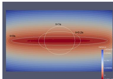
Figure 3: initial distance function field and the obtained interfaces (white lines) at  $t=0s, 0.2s$  and  $1s$  [3]
