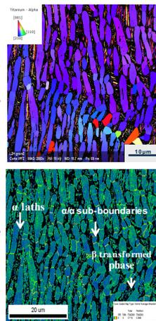
Figure 3: Inverse pole figures map of the  $\alpha$  phase in a Ti-64 sample after 20% deformation at 950°C.
