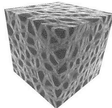
Example of a 3D polycrystal non-conforming FE mesh<sup>b</sup>
